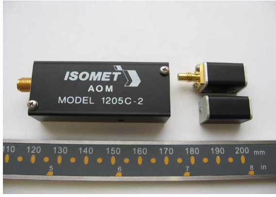
Fig. 4. Photographs of the "ISOMET" 1205-C2 AOM and of the "VNIIFTRI" AOM - RN.
